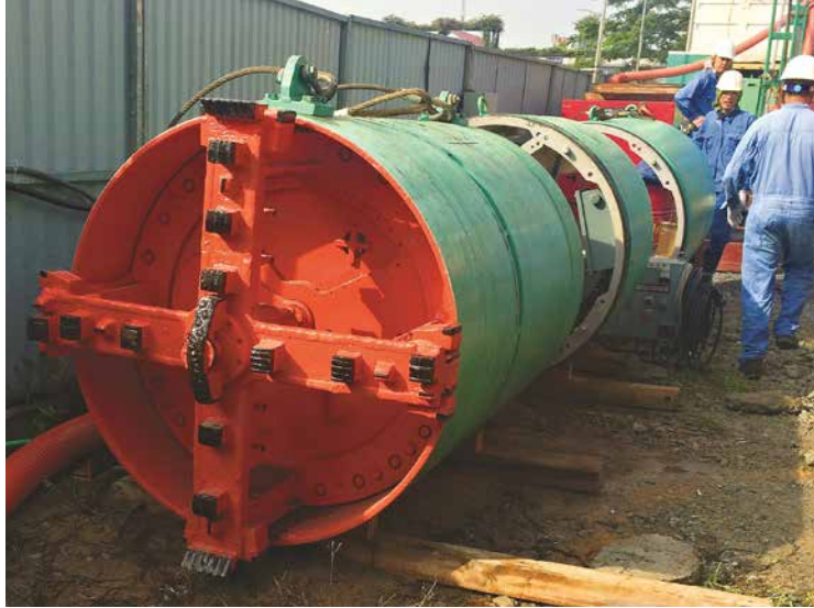
▶ HCMC Water environment improvement (Package G) Pipe jacking construction
